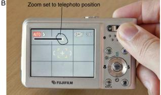
**Figure 8** A, In a compact camera, moving the zoom indicator to the left activates the wide-angle range (to make a nearby subject appear farther away). B, The zoom indicator to the right of the scale indicates the telephoto range (to make a distant subject appear nearer).
