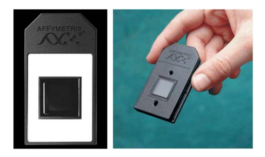
Figure 1. DNA oligonucleotide microarray (Affymetrix, Santa Clara, USA).
