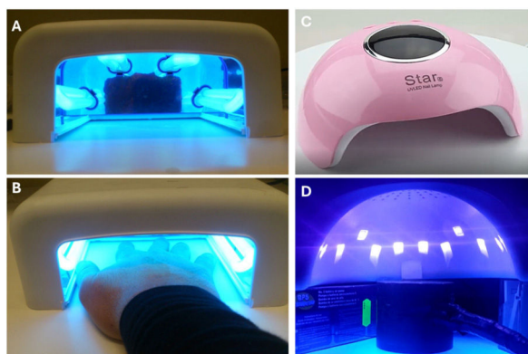
Figure 1 Images of the polymerization lamps used in this study. A) Fluorescent lamp with tube arrangement. B) LED lamp. C) Image of the hand placed to measure the measurement distance (8 cm) under the fluorescents. D) Placement of the sensor to measure the spectral irradiance of the LED lighting source.
