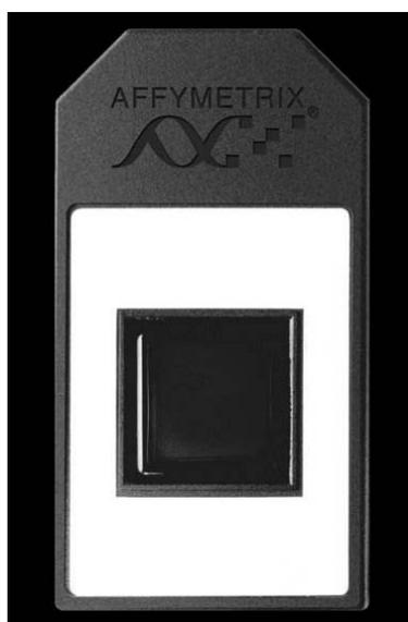
**Figure 1.** DNA oligonucleotide microarray (Affymetrix, Santa Clara, USA).
